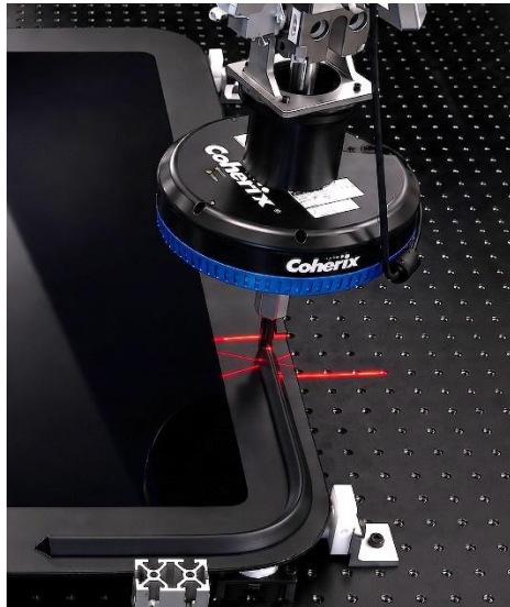
High-speed lasers check the application of adhesives on a vehicle window at the Coherix product development center in Ann Arbor, Michigan.
