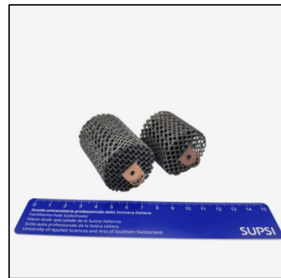
POCS with copper-plated pins (rotated cube unit cell) Cell size: 4 mm Strut size: 1 mm
