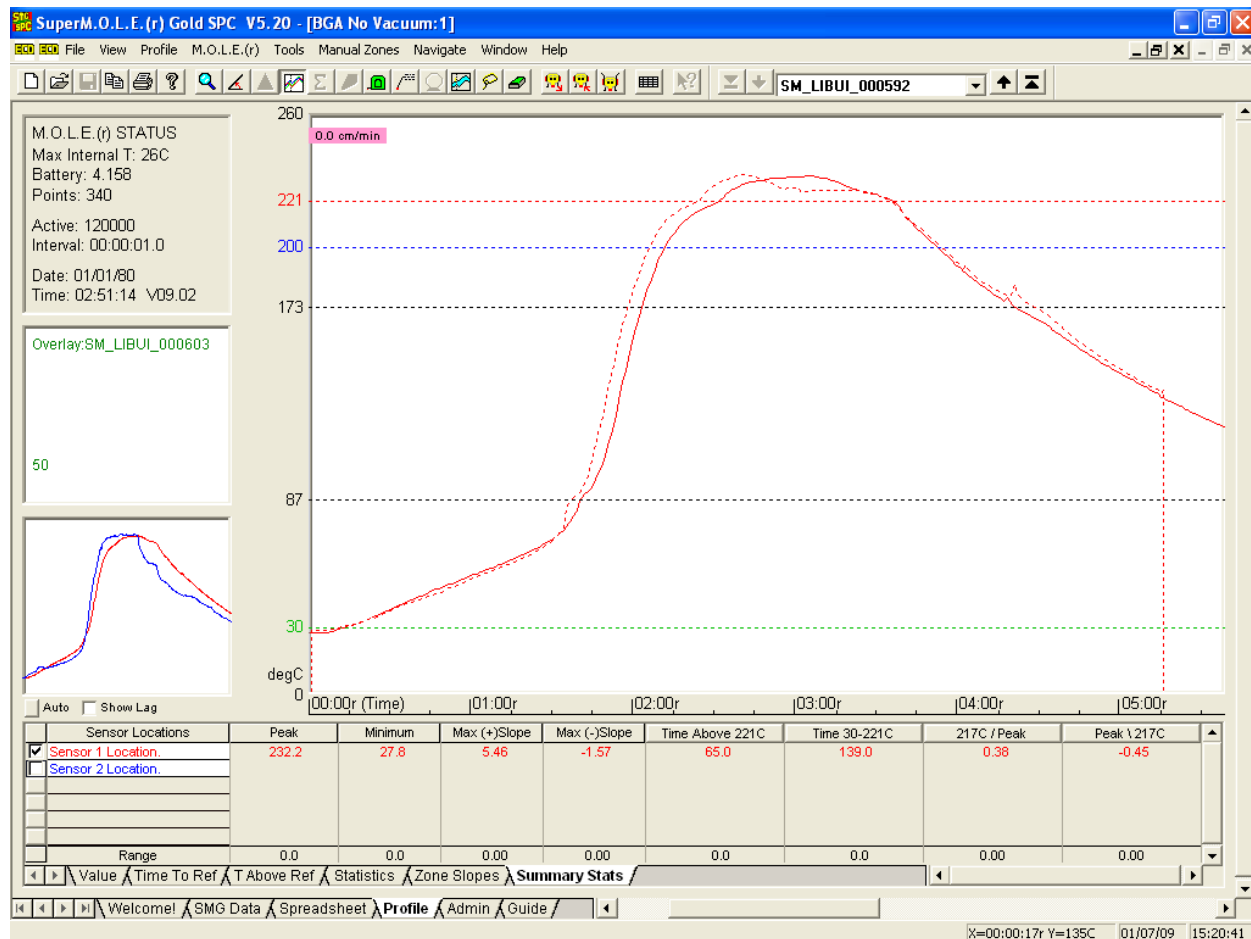
Figure 3 - Solder profiles overlapped: no-vacuum (solid) and with vacuum (dashed)
