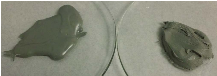
Figure 5 – Fresh Solder Paste (Left). Aged Solder Paste (Right)
