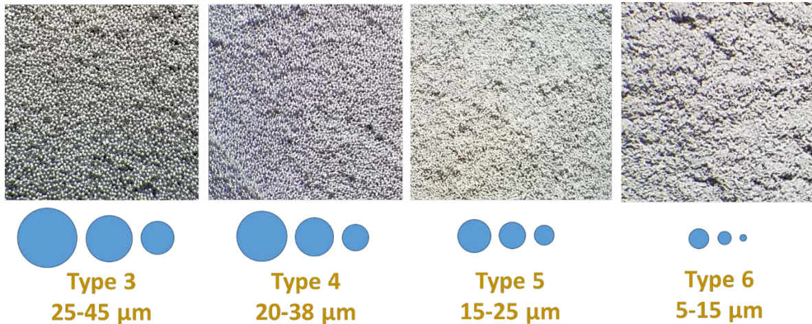
Figure 2 – IPC Type 3, 4, 5 and 6 Solder Powders
