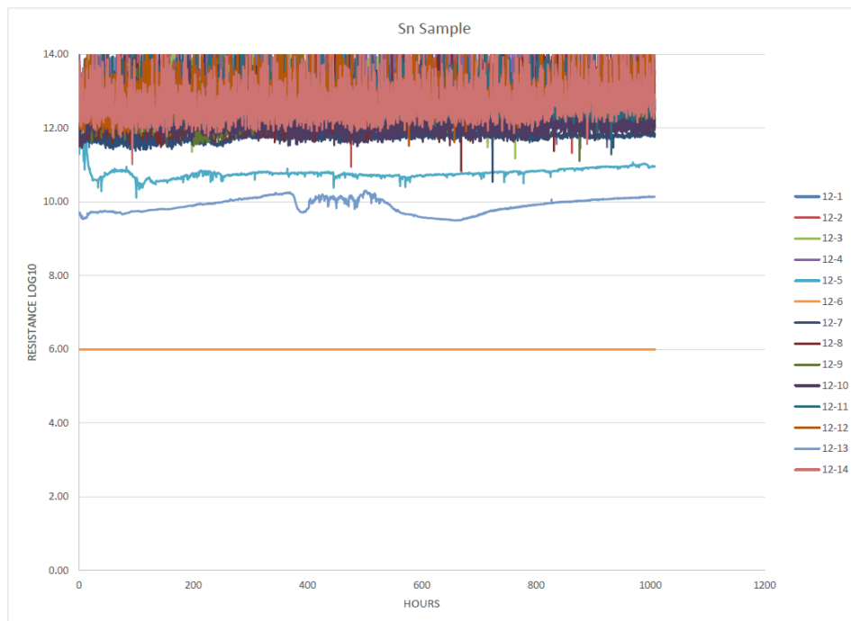
Figure5. Immersion Sn sample 12 SIR with one channel below the resistance limit
