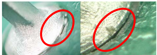
Figure 22: Peeled land after 255C° solder bath (both images are of the same component, zoomed to show detail).
