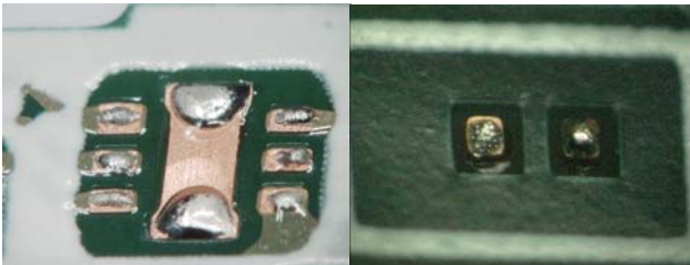
Figure 13: Unmelted solder and insufficient flux (left). Insufficient amount of solder (right).
