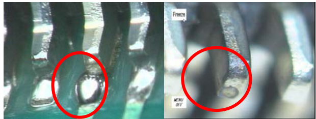
Figure 18: Repelled solder and lead tip oxidation.
