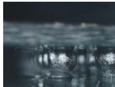
Figure 6: Insufficient melting due to oxidation resulting from flux deterioration. (e.g. due to long pre-heat)
