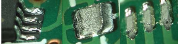
Figure 16: Solder defects captured with the 360° rotational adapter.
