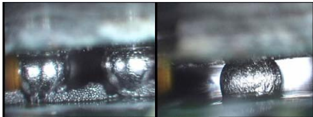
Figure 12: Unmelted solder (left), and corner BGA inspection (right)
