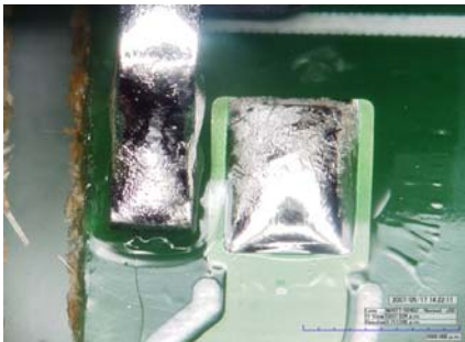
Figure 1A: Spattered flux residue may indicate voids.
