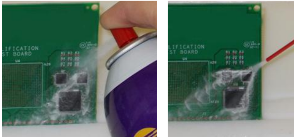
Figure 8: Visual comparison of an aerosol spray without (left) and with a straw attachment.
