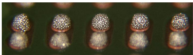
Supplier B (correct copper size)
