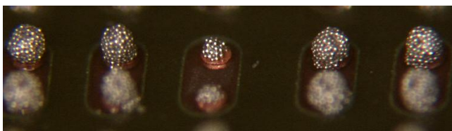
Supplier A (over-etched copper)
