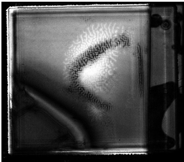
Figure 6: Reflection mode C-Scan of a die attach level deeper in the stack revealing another large void (white area). The shadows from the voids at die attach level one are also present in the image.
