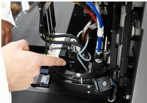
The print head makes all the difference: Coating engineer Kevin Poth points to the centerpiece of the new SUSS LP50 "Pixdro" printer.
