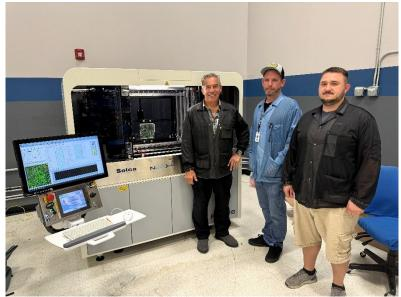
The PILOT V8 NEXT's vertical, dual-sided architecture enables simultaneous probing on both sides of the printed circuit board assembly (PCBA), optimizing efficiency and ensuring comprehensive, accurate test coverage. This dual-sided probing capability significantly enhances productivity while ensuring the high testing standards required for today's advanced electronics manufacturing.
