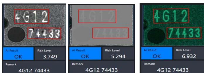
Figure 2. AI-OCR can read markings that otherwise would require visual inspector confirmation.
