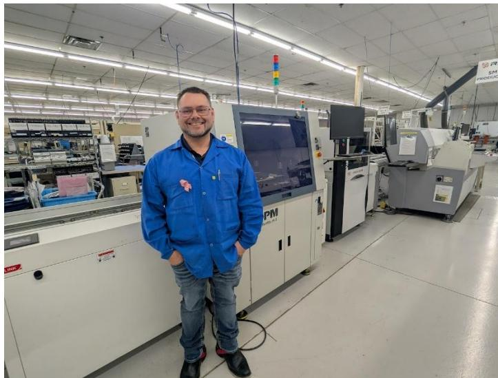
To support its commitment to quality and efficiency, RBB has installed **MPM MOMENTUM II 100 stencil printers** on both SMT lines, offering industry-leading alignment repeatability, wet print accuracy, and dual-lane processing capabilities—all in a compact, space-saving design. Key features of the Momentum II 100 include:
