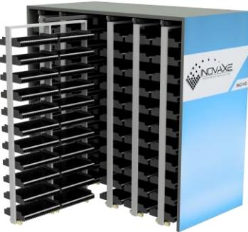
InoHD™ is designed to address one of the most persistent challenges in electronics manufacturing: space. The system removes the need for traditional storage aisles by combining servo-driven mobile shelving with Inovaxe's smart sensing and pick-to-light technology. This approach allows manufacturers to store up to 310 SMT reels per square foot, while still providing fast, guided access and real-time inventory verification.
