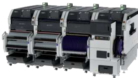
Fuji SMT pick and place machine NXTR S model
