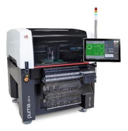
Designed to meet the growing demands of high-mix, low- to mid-volume production, the Puma Ultra All-in-One integrates multiple functions—including Pick & Place, jetting, dispensing, and inspection (2D SPI & 2D AOI) —into one compact and modular platform. This flexible architecture allows manufacturers to scale capabilities over time without the cost or complexity of multiple standalone machines.
