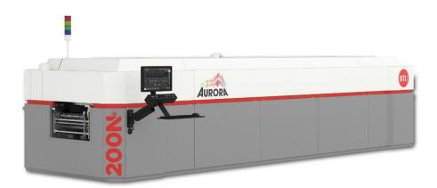
The Aurora 200N is BTU's most advanced reflow oven to date and the longest in the company's history, offering 200 inches of heated length. Its extended configuration supports line speeds up to 25% faster than previous models, helping manufacturers meet high-throughput production goals. Designed with flexibility in mind, the Aurora 200N can be shipped in two modular sections, simplifying delivery and installation without sacrificing performance.
