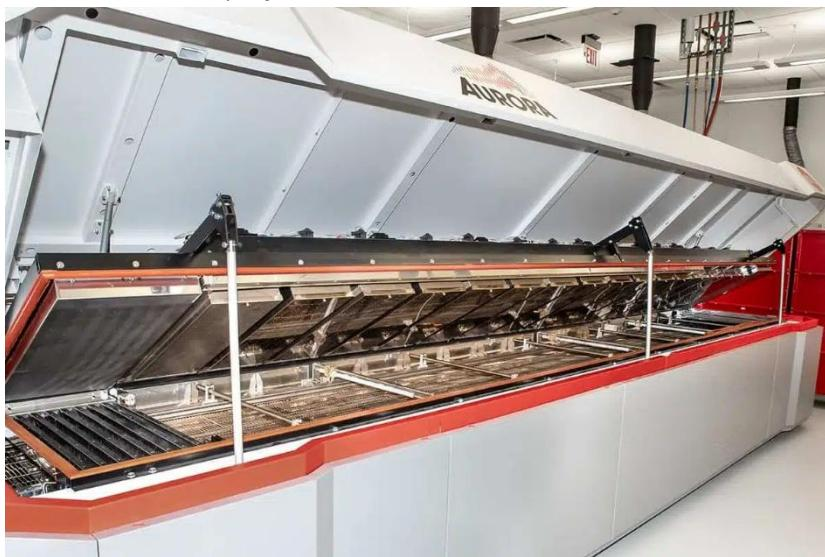
The Aurora platform reflects a clean break from traditional fixed oven designs. Its factory-configurable heating and cooling architecture—a first in the industry—lets users tailor the oven to the exact needs of their product mix, whether that means handling unusually heavy boards, managing sensitive cooling requirements, or pushing throughput on high-volume SMT lines.
