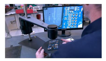
In the fast-paced world of electronics manufacturing, ensuring the precision and quality of printed circuit boards (PCBs) is critical. From quality control to rework on faulty PCBs, the tools you use can significantly impact efficiency and outcomes. This is where the camera microscope, also known as digital microscopes, become indispensable. But why opt for a camera microscope over traditional tools like desk magnifiers or stereo microscopes?
