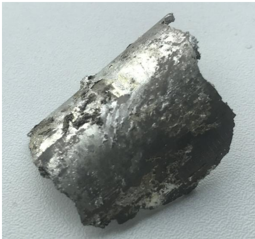
Figure 31. A mixture of dross and needles of alloy E found between inner and outer tube.
