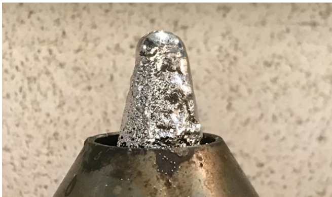
Figure 13. The solidification of the solder at lower temperatures and pump speed.
