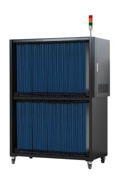
The IMS-100 (T) is a high-resolution barcode camera capable of reading and storing information for up to four 7", one 13", and one 15" reel. The system helps automate your incoming process and makes the relabeling process safe and easy, helping minimize human error.
