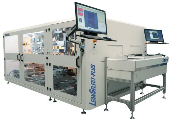
The assemblies are loaded and unloaded via two separate transports on the front. Therefore, the system can be flexibly integrated into any production concept: from manual operation with a simple transverse conveyor, through the individualized, semi-automatic workstation, to integration in a fully automated production line with several workstations.
