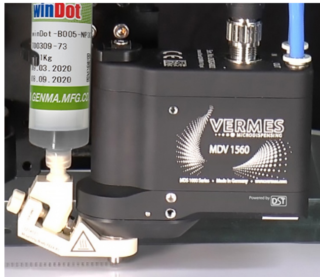
VERMES Microdispensing System MDS 1560 and GENMA winDot solder paste
