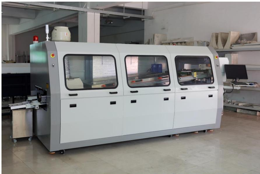
The NRW Series features an automatic solder pot (in/out & up/down), a spray nozzle cleaning system, and even spray for minimized overlapping. The heavy-duty conveyor rail has a robust conveyor finger. Additionally, the system has five individual preheating zones.
