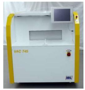
The combination of the vapor phase soldering with a vacuum process significantly increases the reliability of the finished product. Sensitive applications (e.g. fine pitch) mostly require a flexible machine with adjustable vacuum parameters. The VAC745 and VAC765 meet and exceed those requirements with the ability to influence evacuation time, holding time of the vacuum and venting time. Additionally, the patented InVapour Technology creates a fully inert soldering and vacuum process.
