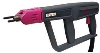
The handheld version of the Atmospheric Plasma System has a unique two-handed nozzle with dual triggers. The first trigger prepares the system for use, while the main trigger activates the plasma nozzle. This system allows hand treatment of large substrate surfaces in nearly any well ventilated environment. The unit features a 16' cable between the power supply and the portable plasma nozzle.
