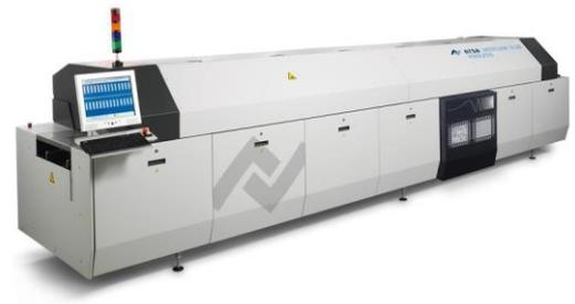
Ersa offers a range of selective solder systems, starting with the Smartflow 2020. Due to its universal pallet fastening, the Smartflow can handle PCB sizes of up to 508 x 508 mm [20" x 20"]. The Smartflow 2020 is smart and compact without compromising quality.
