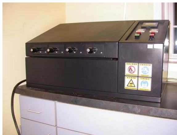
Figure 6: Steam aging apparatus used to stress ENIG and EPIG solder wicking
