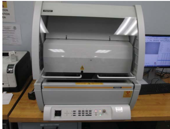
Figure 5: XRF used to measure plate thicknesses of the ENIG and EPIG test samples
