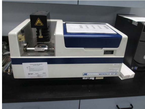
Figure 4: Wetting balance used to test solderability
