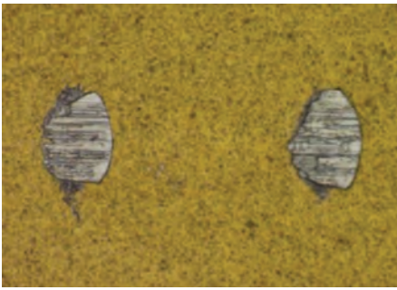
Figure 2. Sheared wire bonds.
