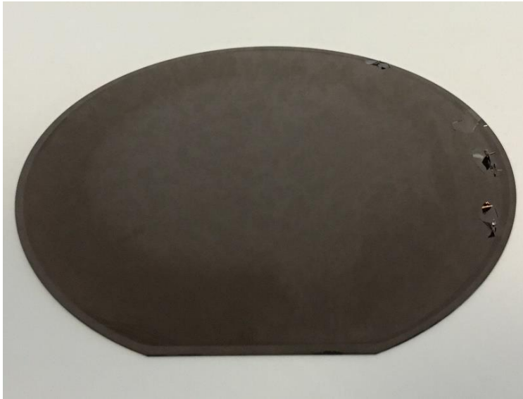
Fig 1 Wafer with known good and bad film adhesion
