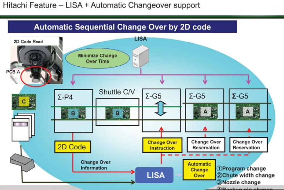
time savings begin to accumulate; automated control of these (Figure 3, above) by LISA now saves 25% of the time previously needed for line changeover.
