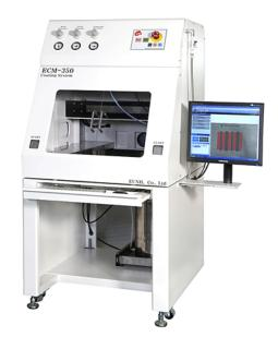
The advantages are that the automated selective coating is good for consistency, producing repeatable results. It increases productivity (high throughput and reduced labor costs), improves material utilization, and improves quality with little to no masking.
