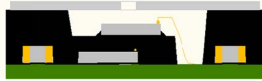
LGA-MCP System-in-package with custom cavity and top port
