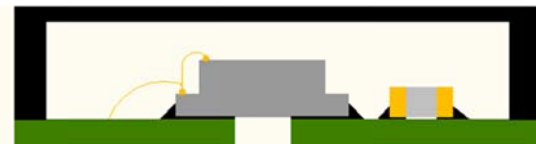
LGA-MLP system-in-package with bottom port
