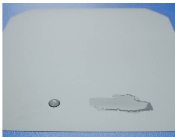
Fig. 3 Water droplet on sawed silicon untreated (left) and treated for 2 s with UV / ozone (right)
