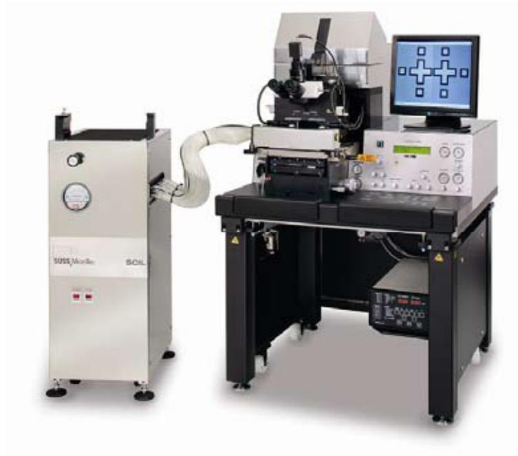
**Figure 3:** Photograph of MA6 mask aligner with SCIL upgrade tooling.
