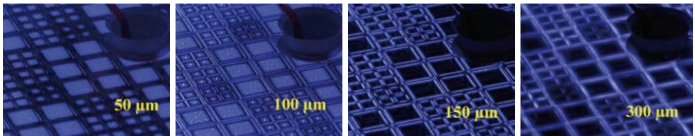
Figure 2: Local plasma treatment (LPT) of a structured silicon wafer surface. The photographs were taken with different distances between the Si wafer and a transparent counter electrode (ITO on glass), as indicated on the photographs. At low distances, the discharge is limited to the recessed areas of the wafer, at large distances it is concentrated on the protruding ridges of the structure.
