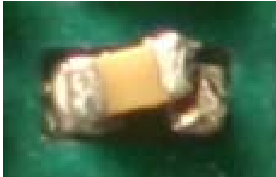
Fig5. Skewed component due to inaccurate placement
