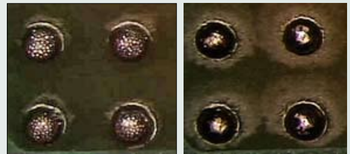
Fig. 5 Bumps with graping (left) and without graping (right).
