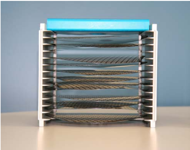
Figure 4. Image showing the large amount of out-of-plane distortion and warpage typical of unsupported ultrathin wafers. In this case approximately 10 mm. Notice also the wide slots in the special cassette designed to accommodate said distortion.
