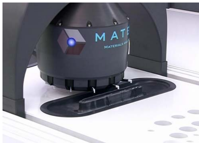
Figure 3. Image of MATECH's side-contact chuck (CAT chuck). Notice the position of the fingers that have moved out of the way to avoid contact with the etching fluid while the remaining fingers stay in contact with the sides of the thin wafer keeping it within capture range of the fluid pool. The adaptive handling allows the chuck to manage ultrathin, severely distorted wafers while making no contact with the non-process side.
