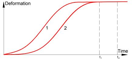
figure 2: Deformation curves seen on a bonder without deformation control
