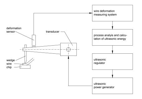
figure 3: Bond process control for aluminium wire bonders
