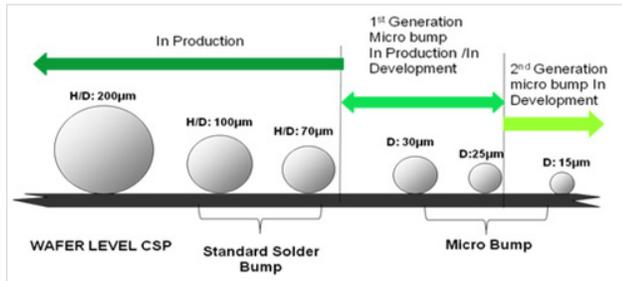
Figure 1 - Shows the different bump sizes currently in production and in development
