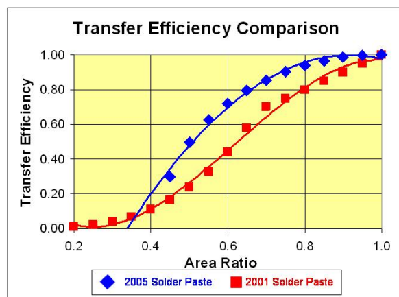
Figure 8. Transfer efficiency comparison of different solder pastes. Notice the newer paste shows better release characteristics throughout the entire area ratio range that was measured (0.4 to 1.0).
