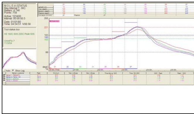
Figure 5. Soak profile for Tin-Lead alloy. Soak time is 60 seconds at 160 C. Peak temperature is 210-220 C.
