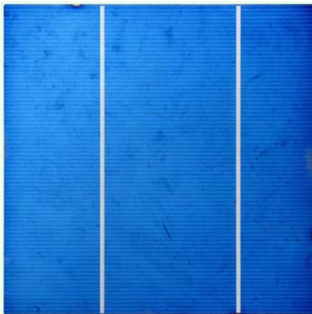
Figure 4: As-Printed Silicon Wafer with collector lines and bus bars. Collector and bus lines were printed in separate steps using a multi-nozzle print head and a bus bar printing head.
