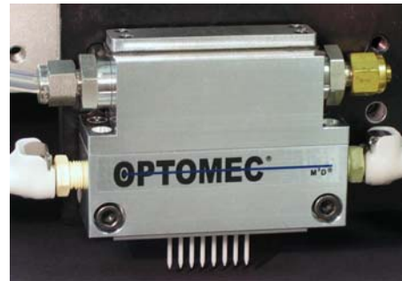
Figure 3: Multi-Nozzle Print Head. The Aerosol enters a manifold at the top of the Print Head and is distributed evenly among all nozzles.
