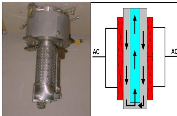
Figure 3: Electromagnetic solder pump
