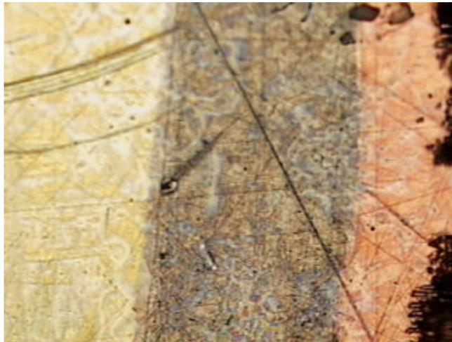
*Figure 11: Complete wetting post mechanical stress*
