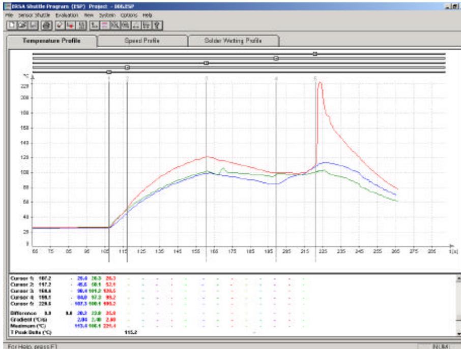
Figure 5: Selective soldering thermal profile
