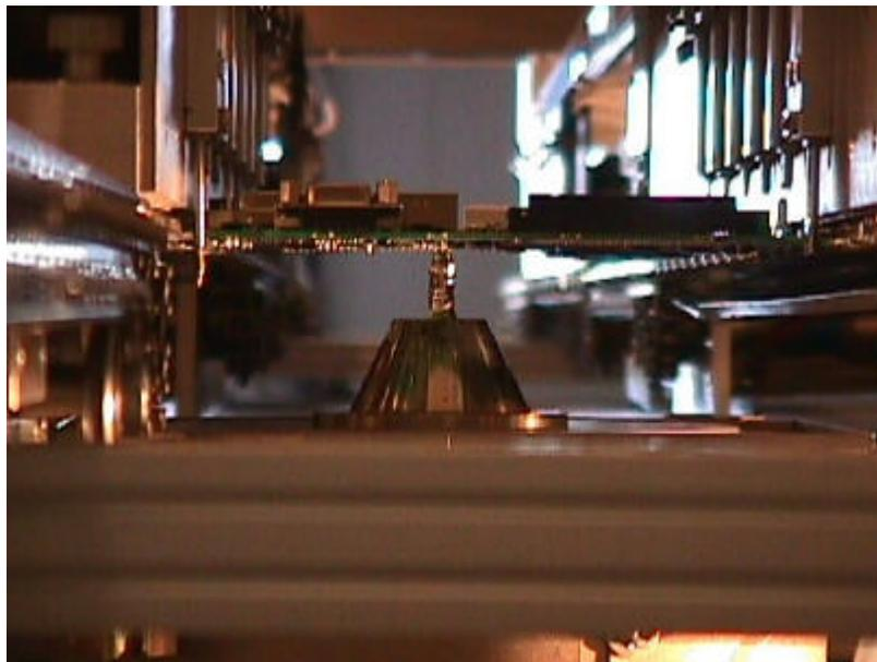
*Figure 4: Programmable selective soldering system*
