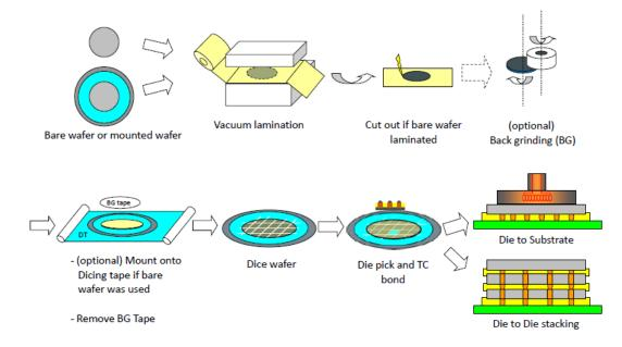
The latest NCF material to be introduced to market is a 2-in-1 wafer-applied underfill film from Henkel. Henkel's NCF has been developed to facilitate die processing for die that are less than 60  $\mu$ m thick and, as compared to previous generation materials, the new NCF has a long work life of 8 weeks; 6 weeks with the backgrinding tape and an additional 2 weeks once the
