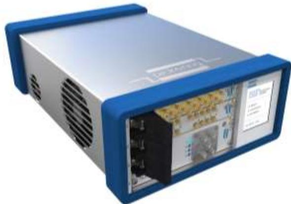
**High-Density Modular LXI Ethernet Reed Relay Matrix** – Originally designed to test Semiconductors at wafer and package levels, this Reed Relay Matrix solution combines our LXI Modular Matrix Chassis with our new plug-in matrix modules that provide access to all signal connections on 200 pin connectors. The range includes four models covering matrices of up to 1,536x4 in increments of 128, 768x8 in increments of 64, 384x16 in increments of 32, and 192x32 in increments of 32.
