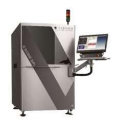
In SMT electronic assembly production, 3D solder paste print inspection has established itself as the additional inspection gate to complement optical or X-ray inspection of electronic assemblies. The key task of the 3D SPI is detecting impermissible printed pads in terms of volume, form, smearing, paste bridges and offset.
