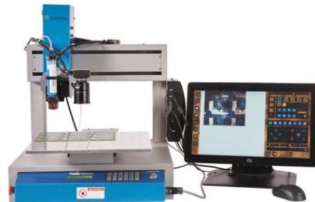
The [TS5000DMP-DCX](#) is a disposable material path rotary valve equipped with a quick access hinged door, for rapid feed-path replacement. Techcon's patented Disposable Material Path (DMP) valve contains a disposable feed screw for easy maintenance and reliable dispensing. With the feed screw made of Delrin®, the valve is designed for use with two-compound and UV fluids.
