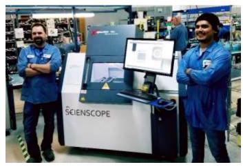
The X-SPECTION 6000 systems have been setup and programmed to perform automated inspection of BGAs. Milwaukee Electronics uses them to check the first product off the line daily. The company also operates a quick turn operation in Oregon named Screaming Circuits that offers rapid turnaround assembly and prototyping. The X-SPECTION 6000 also is used to evaluate Milwaukee Electronics prototypes and validate their process for the rapid turnaround products.
